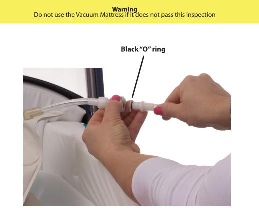
Connect the two sections of tubing until an audible "click" is heard and the black "O" ring disappears from view. This opens the valve, allowing air to be removed from the mattress via suction.
